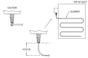
Figure 1: Install capillary in horizontal pattern only
